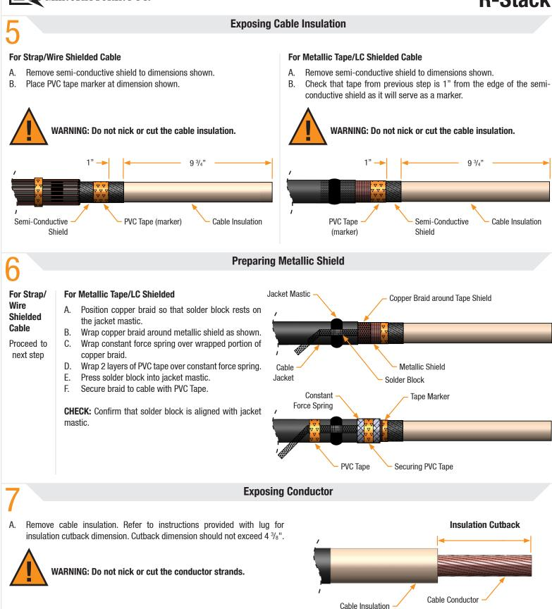
NOTE: Confirm all dimensions with To-Scale Cable Cutback Template before proceeding.
