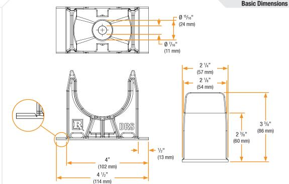
Tabs on both sides control spacing between saddled components. Designed to break easily at the "V" notch on both ends if necessary.
