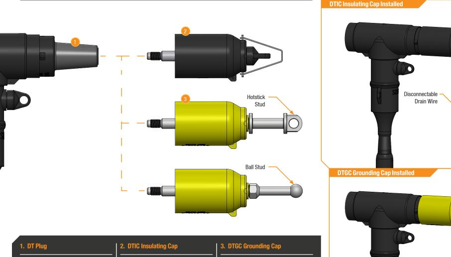
This plug features an IEEE 386 standard deadbreak interface on one side and our innovative DT Interface on the other. The DT Plug can be installed on the backside of Deadbreak Elbows, Bushing Extenders, or other accessory to provide a convenient grounding location.
