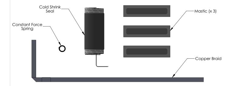
Richards Cold Shrink Shield Kit provides an easy way to ground and seal metallic shielded cable when installing Richards premolded equipment incuding elbows, T-bodies, and splices. The kits can be used with Loadbreak and Deadbreak equipment at 600A for 15kV, 25kV, and 35 kV Voltage classes.
