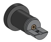
Richards 15/25/28kV Copper Straight Receptacle Adapter Kit converts a 900A interface (IEEE 386 Fig 11) to a disconnectable splice interface for connection to a joint sleeve (P625JS).
