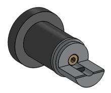
Richards 15/25/28kV Straight Receptacle Adapter Kit converts a 600A interface (IEEE 386 Fig 11) to a disconnectable splice interface for connection to a joint sleeve (P625JS).
