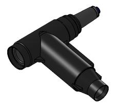
Richards 25/28 kV R-800 (628MN) is a 15/25kV 600A elbow with a 25kV 200A loadbreak tap molded into the body. This combination design reduces the number of components, time, and effort required for installation.
