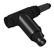
Richards 25/28kV R-800 (628FT) is a 15/25kV 600A elbow with a 25kV 200A loadbreak tap molded into the body. This combination design reduces the number of components, time, and effort required for installation.
