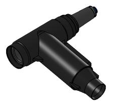
Richards 25/28 kV R-800 (628FN) is a 15/25kV 600A elbow with a 25kV 200A loadbreak tap molded into the body. This combination design reduces the number of components, time, and effort required for installation.
