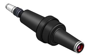
Richards 15kV Loadbreak Reducing Tap Plug (P615LRTP) converts a 15/25kV 600A deadbreak intérface (IEEE 386 Fig. 11) to a 15kV 200A loadbreak interface (IEEE 386 Fig. 5) for use with a loadbreak elbow or cap.
