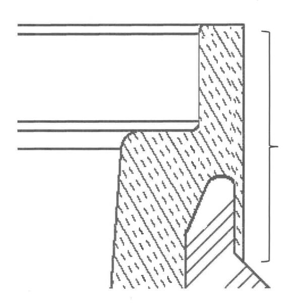
Length of insulation overlap in this region dictated by shield break electrical requirements
