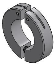
Richards Disconnectable Joint Retaining Rings are used to prevent movement of Deadbreak Cable Adapters during installation of the Joint Sleeve. This accessory is made from tin plated aluminum and sized based on conductor.
