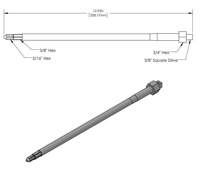
The P6AT is an installation tool for use on Medium Voltage Cable Accessories 15kV through 35kV. Equipped with a dual 5/16" and 3/8" hex tip, the P6AT can be used to install a wide variety of accessories. The back of the P6AT features both a 3/8" square drive and a 3/4" hex for compatibility with multiple torque-driving tools.
