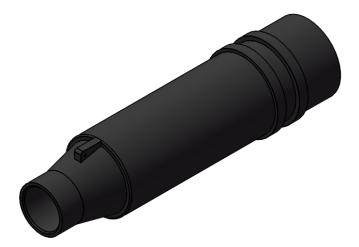
Richards Disconnectable Joints provide a robust, versatile option for splicing underground medium voltage cables. They can be used for straight or multi-way splicing and can be disconnected for circuit isolation, grounding, expansion and more. Disconnectable Joints are molded from peroxide-cured EPDM and are fully shielded and submersible.
