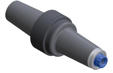
Richards 25kV Loadbreak Elbow Tap Plug (P625ETP) converts a 15/25kV 600A Deadbreak interface (IEEE 386 Fig. 11) to a 25kV 200A Loadbreak interface (IEEE 386 Fig. 7) for use with a Loadbreak elbow or cap.
