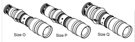
Richards Disconnectable Joints provide a robust, versatile option for splicing underground medium voltage cables. They can be used for straight or multi-way splicing and can be disconnected for circuit isolation, grounding, expansion and more. Disconnectable Joints are molded from peroxide-cured EPDM and are fully shielded and submersible.
