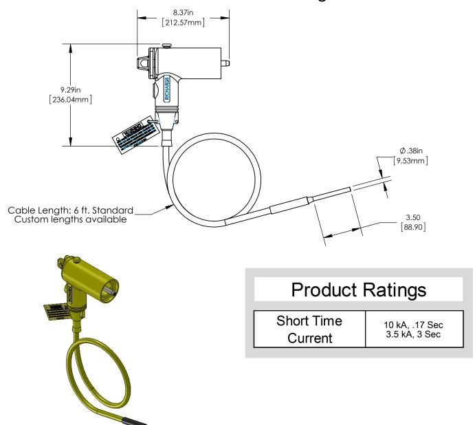
Richards 200A Loadbreak Connectors provide an easy way to connect or disconnect energized power cables from equipment at 15 kV.
