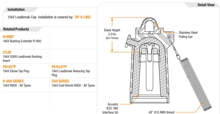
48" #12 AWG tinned copper drain wire
