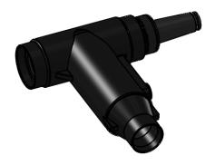
Richards 15 kV R800 (618MT) is a 600A elbow with a 200A loadbreak tap molded into the body. This combination design reduces the number of components, time, and effort required for installation.
