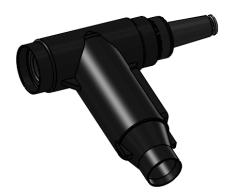
Richards 15 kV R800 (618MN) is a 600A elbow with a 200A loadbreak tap molded into the body. This combination design reduces the number of components, time, and effort required for installation.
