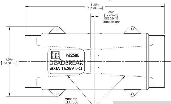
Fig. 11 Interface on both sides
