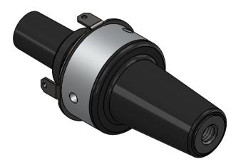
Richards 15/25 kV Reducing Tap Plug (P925RTP) converts a 900A interface (IEEE 386 Fig 11) to a 200A deadbreak interface (IEEE 386 Fig 4) for use with a 200A deadbreak elbow or cap.
