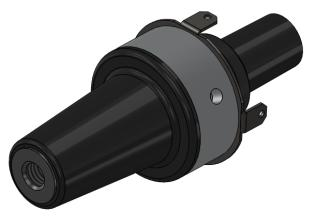
Richards 15/25 kV Reducing Tap Plug (P625RTP) converts a 600A interface (IEEE 386 Fig 11) to a 200A deadbreak interface (IEEE 386 Fig 4) for use with a 200A deadbreak elbow or cap.
