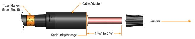
**CHECK:** Confirm that edge of tape marker is flush with end of cable adapter as shown.
