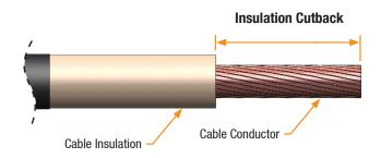
**NOTE:** Confirm all dimensions with To-Scale Cable Cutback Template before proceeding.
