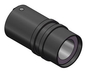
Richards 15/25/28kV Insulating Cap (P625JIC) provides a means for shielding, sealing and insulating 600A Disconnectable Joint Bus interfaces that are not in use. The P625JIC is supplied with a stainless steel bail which secures the Insulating Cap to the Disconnectable Joint Bus.
